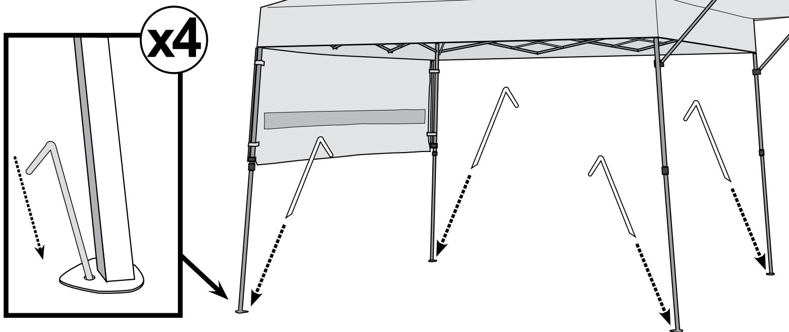
**CAUTION:** Temporary stake anchors are NOT designed for permanent installation. Never leave canopy unattended. For additional important information about anchoring, see next page.
